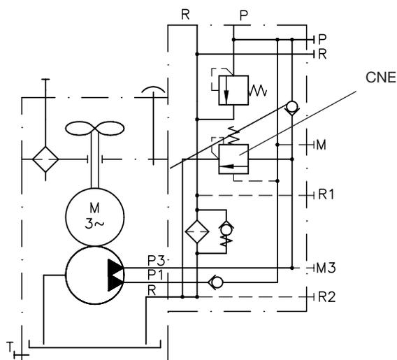
Circulation valve integrated in connection block type AN 21 F2 for compact hydraulic power packs type HK with two pump circuits
