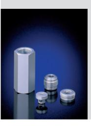
Type BC can be installed in both flow directions. The incorporated check valve is spring loaded. The mounting hole may be shaped with a simple drill (point angle 118°). The orifice inserts, type EB, can be installed in the P-ports of indiv. sub-plate mounted directional valves.
